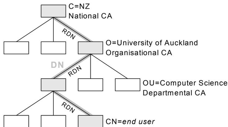
Top-level CA is called the root CA, a.k.a. “the single point of failure”
